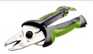
Rapid Fence Plier FP20, Blister, wire fencing plier suitable for securing fencing around large properties or for building animal cages, or protection for young plants, ideal for fixing wire netting to fence wire. Easy to use magazine free operation, for use with Rapid fence hog rings VR16 and VR22, closing diameter for VR16 is 2-8mm, for VR22 is 5-11mm.
