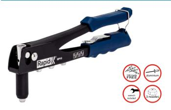
Rapid Hand Riveter RP10, includes a nozzle changing wrench+nozzles, and 100 Rivets Kit (25 of each size 3,2x8mm, 4x10mm, 4x14mm, 4,8x12mm), blister, for use with Rapid 3.2/ 4/ 4.8mm diameter aluminium rivets. Ideal for joining two pieces of sheet metal, plastic, vinyl, leather or canvas together or decorative applications.
